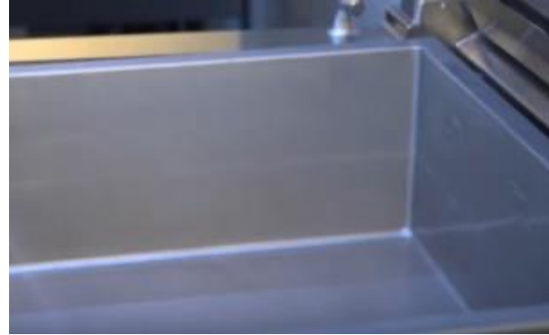
Tank in compound not sticking
