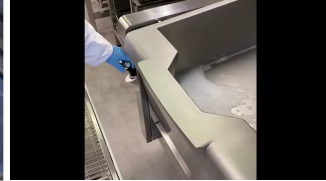
Precipan has an integrated shower and a peripheral gutter that drains up to 82% of the washing water; no risk of water infiltration or flooded soil
