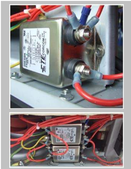
Top: one filter unit (1000W e2s variant) Bottom: two filter units (2000W e2s variant)
